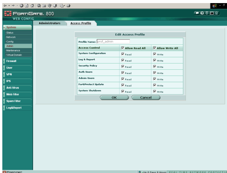
Figure 4 - FortiGate: Configuring User Access Profiles
